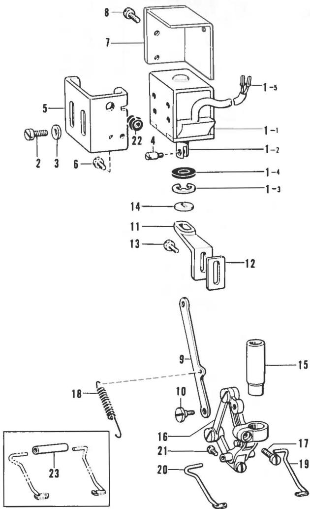
**P. Quick reverse switch mechanism [-400A..-700A..-900A]**
