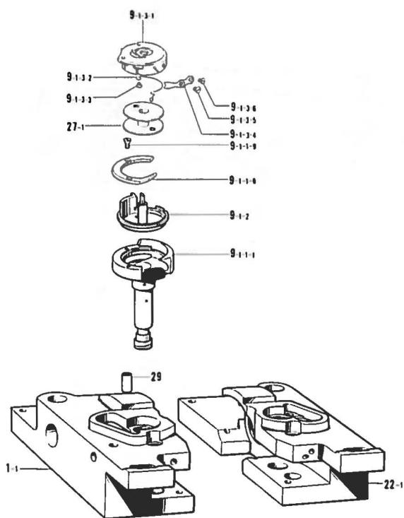
**K. Rotary hook mechanism (3)[-400A--700A--900A]**
